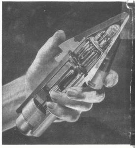
FIVE-TUBE RADIO transmitter and receiver, in the nose of the shell, is the heart of the secret weapon. In flight the transmitter broadcasts a continuous radio wave. Reflected back from the target, this wave explodes the shell at exactly the right moment!
